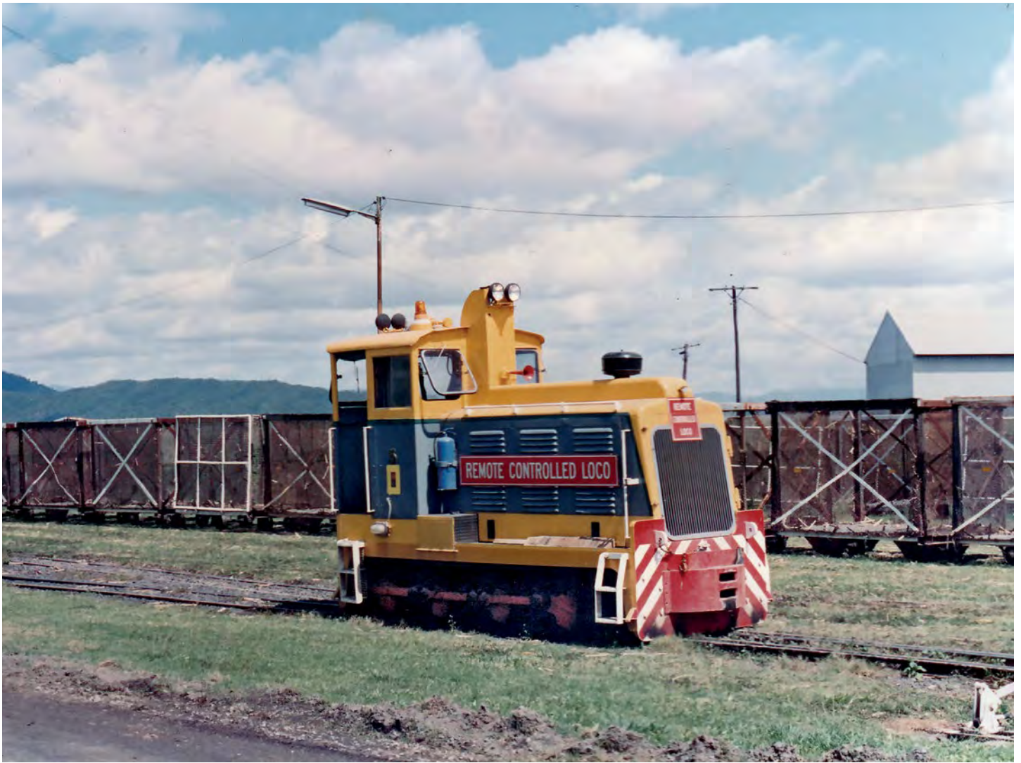
Mourilyan mill No.5 Clyde DHI-71 (B/No.66-491 of 1966) fitted with Theimeg remote control equipment, pictured in the mill yard in 1993. This was the first locomotive to be fitted with this type of control equipment and SRI was heavily involved in this trial. Photo: Chris Hart
